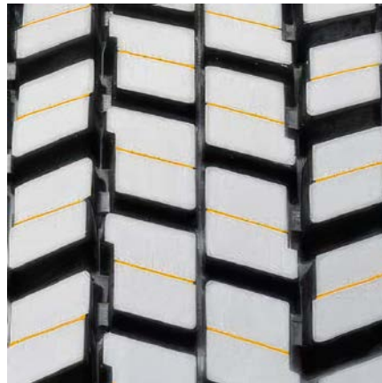
Angled lug design improves overall traction and wet grip.
