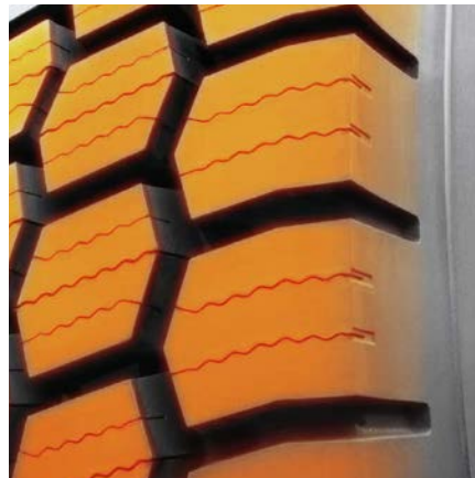
Aggressive tread blocks for outstanding snow and mud handling.
