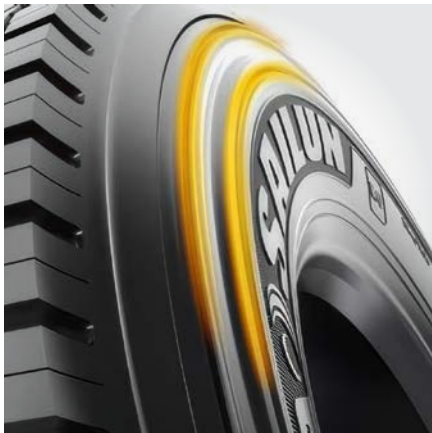
Sidewall protector ribs offer curb abrasion resistance.
