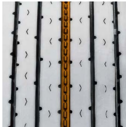
Main groove stone ejectors protect tire against stone drilling.
