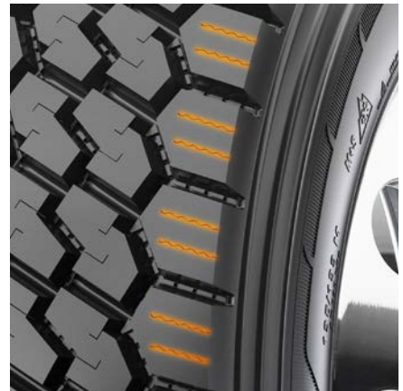
Shoulder block sipes for enhanced ice and snow traction.
