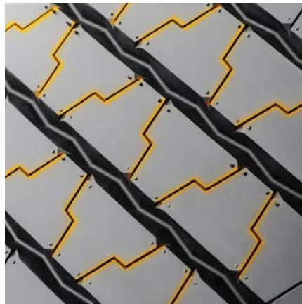
Tread Sipes - Provide extra grip in wet conditions.
