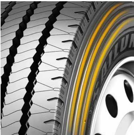
Sidewall protection to resist curb scrubbing.
