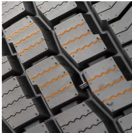
Extensive sipes in tread pattern for increased traction on wet, slush, snow and ice.
