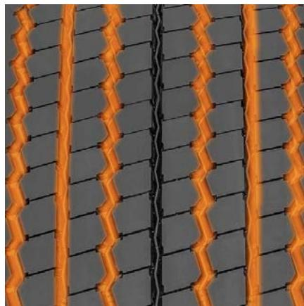
Zig-zag circumferential grooves provide additional biting edges for increased traction.
