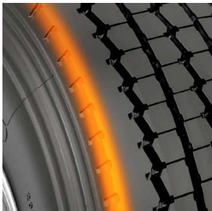
Solid shoulder resists lateral scrubbing in tandem drive axles.
