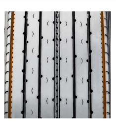
Decoupling grooves help minimize irregular wear.
