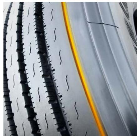
Decoupling groove helps to minimize irregular wear.
