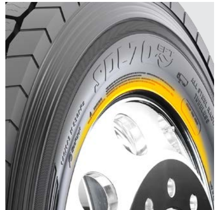
"Slim bead" for reduced rolling resistance.
