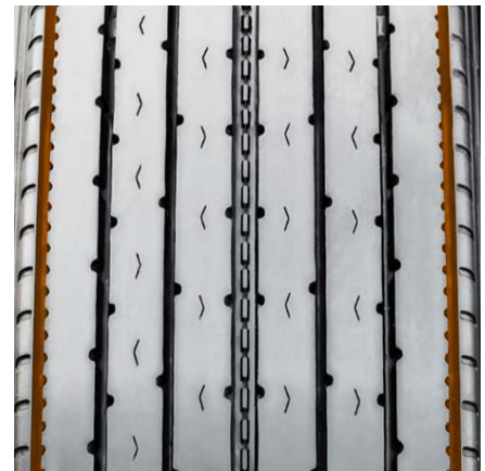
Decoupling grooves help minimize irregular wear.
