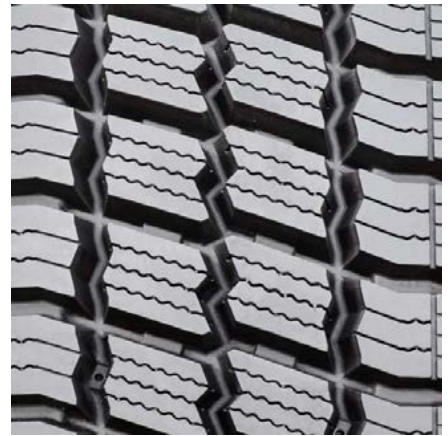
Open tread pattern cleans out well in snow and mud conditions.
