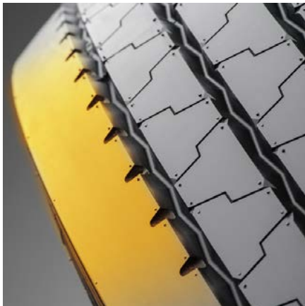
Wide Shoulder - provides stability in lateral scrub situations.
