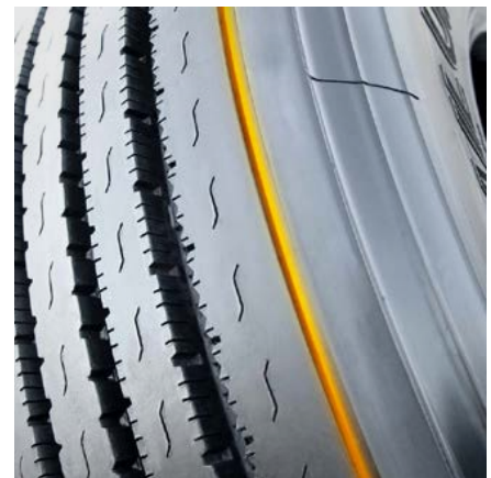
Decoupling groove helps to minimize irregular wear.
