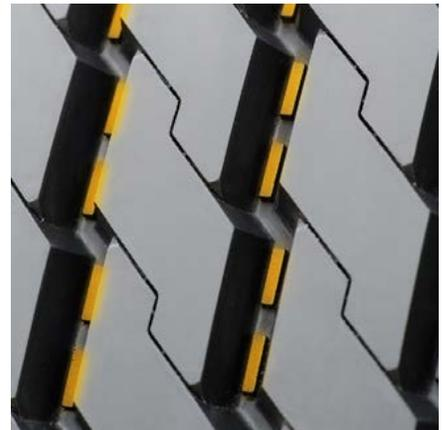
Stone ejectors protect tire against stone drilling.
