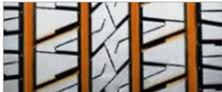
Circumferential Grooves and lateral sipes for increased traction on wet surfaces.
