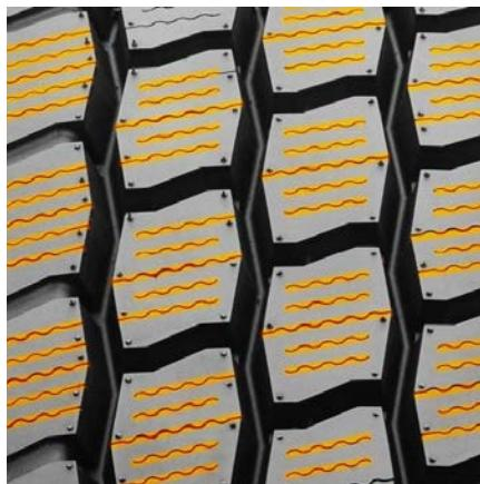
Extensive sipes improve traction in wet conditions and dissipate heat for prolonged tread life.
