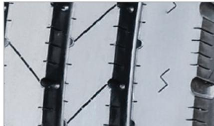
Shallow tread designed to reduce rolling resistance for improved fuel economy. Solid shoulder to resist irregular wear and improve fuel efficiency.
