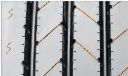
Multi-sipes improve traction in wet conditions and dissipate heat for prolonged tread life.
