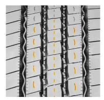
Variable tread angles for self-cleaning and stone ejection.
