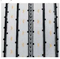
Main groove stone ejectors protect tire against stone drilling.
