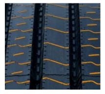
Stone ejectors protect tire from stone drilling.
