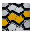
The Sailun S917 drive tire has been engineered to perform in demanding off-road conditions, such as mining, construction and logging applications. The S917 features an aggressive multilug tread design for exceptional off-road traction and an enhanced rubber compound to resist cuts and chunking. Open shoulder ribs deliver superior stability and resistance to uneven wear. The S917's deep 31/32" tread depth provides long tread life and an exceptional cost per mile.
