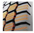
The Sailun SW01 is a premium regional and highway drive tire designed for four-season traction. This versatile tire is ideal for all weather conditions and features an aggressive symmetrical tread design for exceptional traction in mud, snow and ice conditions.
