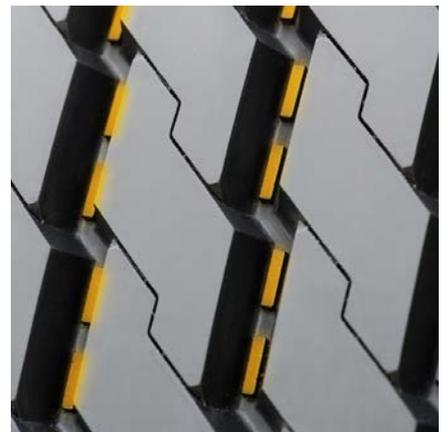
Stone ejectors protect tire against stone drilling.
