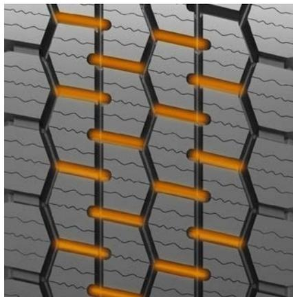
Lug configuration and siping design improves overall snow, ice and wet grip.
