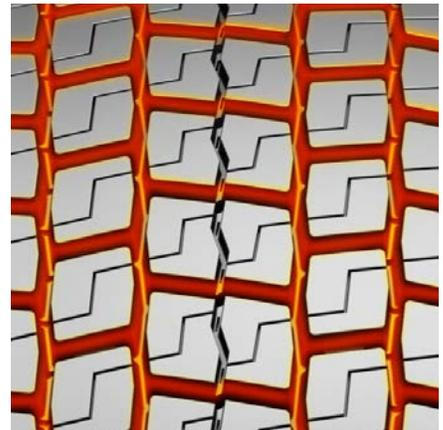
Lug-to-void ratio optimized for self-cleaning and excellent traction.
