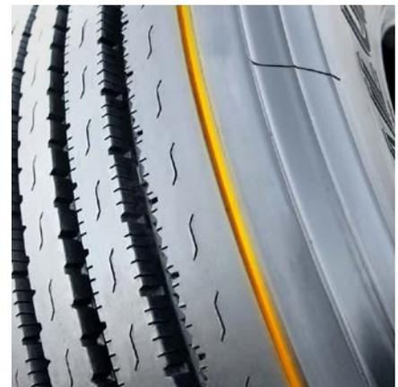
Decoupling groove helps to minimize irregular wear.
