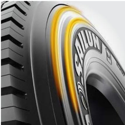
Sidewall protector ribs offer curb abrasion resistance.
