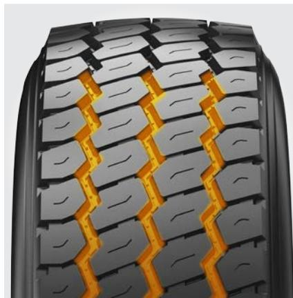
Stone ejectors protect tire against stone drilling.
