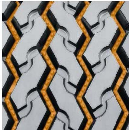
Stone ejectors protect tire against stone drilling.
