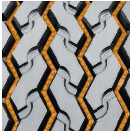
Stone ejectors protect tire against stone drilling.
